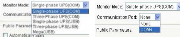
**Communication port:** Communication port only chose the monitoring mode to serial port connection to be checked , if the connection at this time have good connection, communication port can automatically detect the serial number, choose directly. When choosing the USB connection mode software will automatically find the connection, don't need to be set manually. As shown in figure: select single-phase serial connection to choose corresponding communication port.
