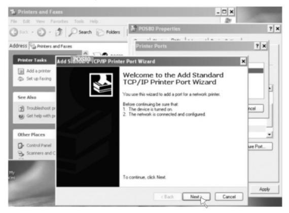
5) according to self-test print of bill IP address enter IP, and then click
